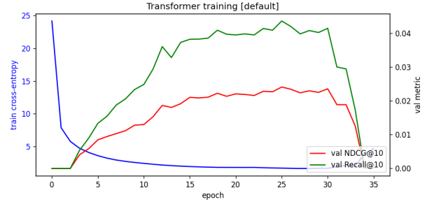
Figure 2: Default-config Transformer training on Colab T4. Train cross-entropy (blue, left axis) decreases monotonically; val NDCG@10 (red) and Recall@10 (green) climb to a peak around epoch 25 and then drift down, after which early stopping ends the run at epoch 33.
